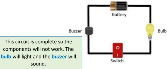
**Components** must be connected in a loop so that electricity can flow. The **electricity flows** through each component in a single pathway.
