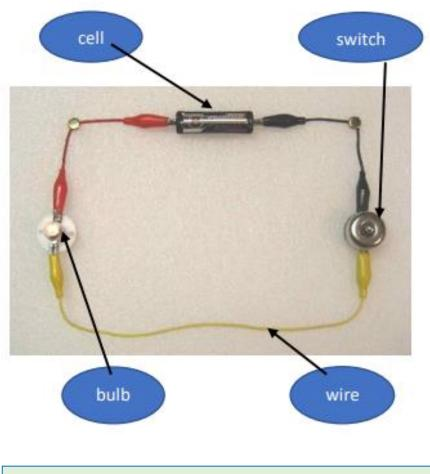
When a **switch** is open (off), there is a gap in the circuit. Electricity cannot travel around the circuit.
